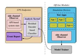
Fig. 1: The general architecture of SideNet.
