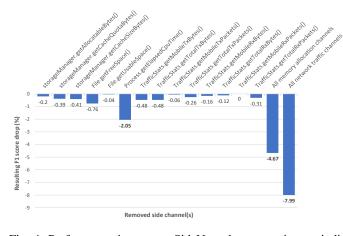
Fig. 4: Performance impact on SideNet when removing an individual side channel (group).
